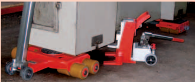
Castors with ball bearings guarantee easy movement
